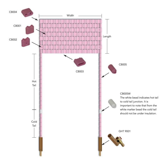
Flexible ceramic pad heating elements are the key item of any localised heat treatment process. They are applied directly to the workpiece to be heated and are held securely in place by means of stainless-steel banding (or soft iron tie wire where only a few heating elements are in the heater band). The heating elements flexibility provides an efficient and high level of heat transfer to the surface being heated.
